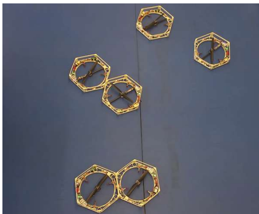
Figure 3.1: Six modules are currently in the process of docking to their partner. One pair has already successfully docked and one is about to dock, whereas the third pair is still separated. Those two are currently approaching each other and will eventually also dock. Once every module has paired up, the process is completed.
